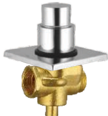
ALC 141 | Metropole Conc. Flush Valve 40mm (1½") with Square Flange with Upper Parts In 1.5" F x Out 1.25" M
