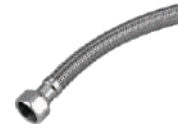
HT 173 | Connection Tube 12 X 375mm (15 ") F 1/2 X F 1/2 Epdm Ss 304 Brass Nut M.R.P. ₹ : 225
