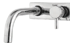
FR 09 134 | Upper Parts Kit for Con. Basin Spout Single. W/M 3/4 Ass. (Consisting of Operating Lever, Wall Flange with Seal, Nipple & Basin Spout) Suitable for ALC-134 M.R.P. ₹ : 2245
